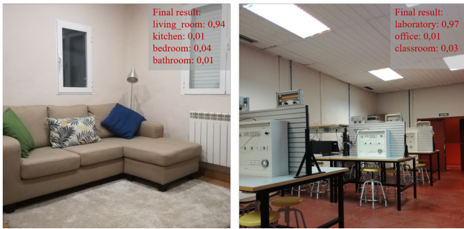
Fig. 1: Example of the results of the proposed multi-classifier model. Two different scenes can be observed, a living room and a laboratory. The model fuses the outcomes of the base classifiers through a weighted voting scheme to give the final prediction about the place that the robot perceives.
